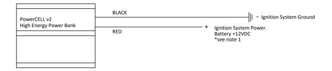
NOTE 1 - Can be connected directly to battery +.
