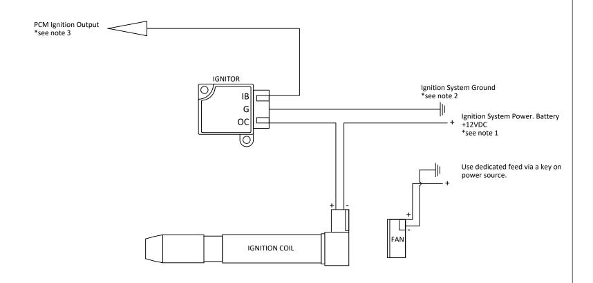
NOTE 1 - Connect to battery post or alternator power cable. Wire in 40 amp relay to switch ignition energy on during keystart.
