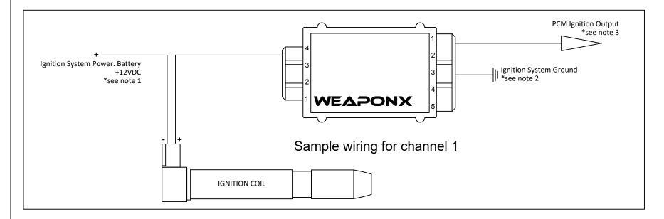
NOTE 1 - Connect to battery post or alternator power cable. Wire in WeaponX 40 amp relay to switch ignition energy on during keystart.
