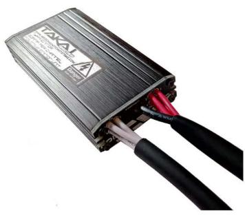
The IGN84XC Ignition Module is available in one to four channel configurations, are 30 amperes per chanel, for use with most inductive two pin ignition coils in 12 or 24\* volt environments.
