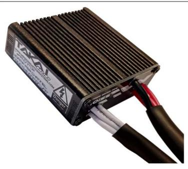
The IGN84X Ignition Module is available in one to four channel configurations, are 30 amperes per chanel, for use with most inductive two pin ignition coils in 12 or 24\* volt environments.
